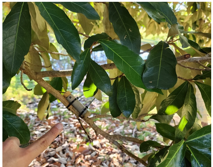
Fig. 2 iButtons are secured inside a protective copper tube and deployed in the study area.
